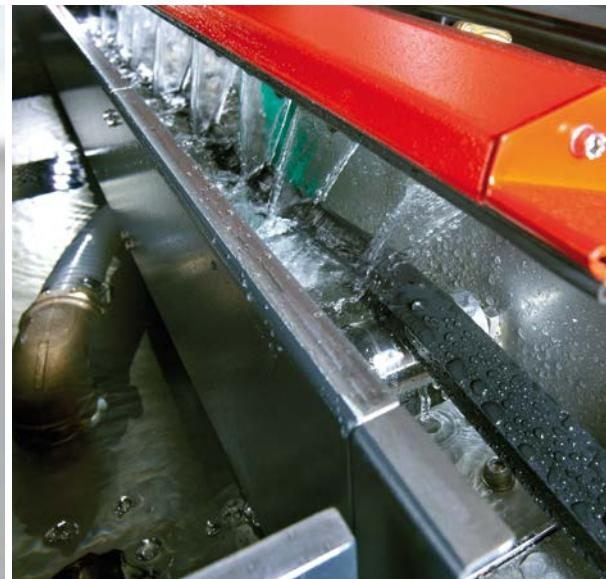
Specially developed flush nozzles, characterize our cooling channel Type 179. The uninterrupted flow of water ensures cooling, even with extremely dirty and hard water.
